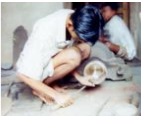
Polishing is mostly done on the inside of bell-metal ware
