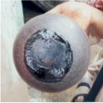
Application of coal tar at the bottom of the ware
