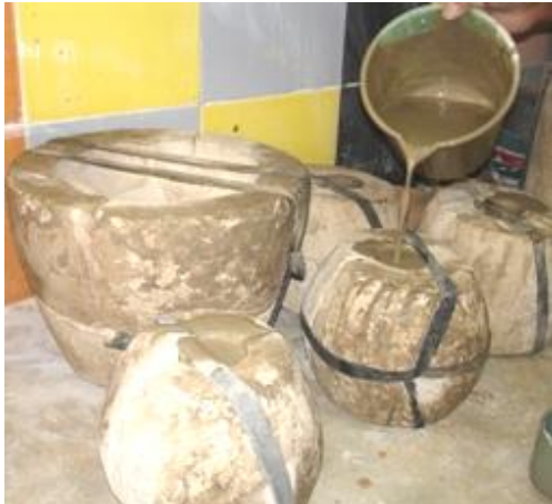
Photograph 7: Molding the clay mixture
