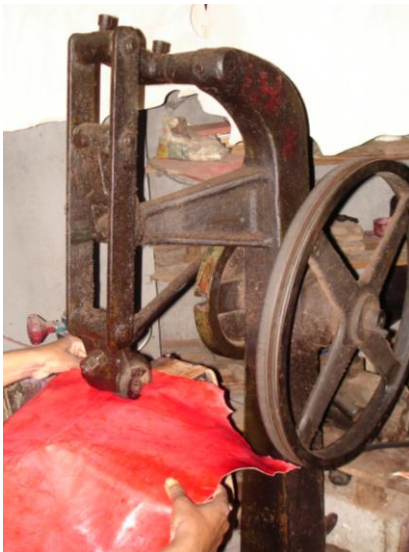
Photograph 3: Embossing the leather using ball press m/c
