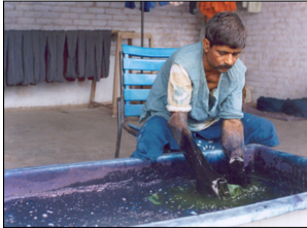
(Photograph Process 4: Preparing the dye bath for indigo dyeing. The cloth is submerged in the bath for approximately 45 minutes.)
