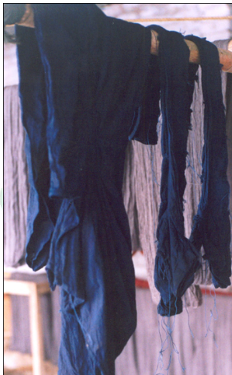
(Photograph product 4: The cloth is left to dry. The indigo dye gets oxidized during this period, leaving the cloth with indigo color.)
