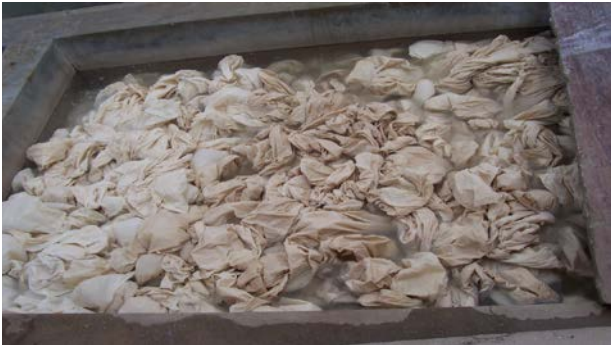
[Photograph 6: Fabric to be printed is washed]
