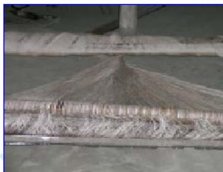
This process starts from one end of the cylinder and goes on till the entire cylinder is covered with thread. *Tora* oil is applied on the threads, to make them move easily on the loom. Once this is achieved, the log upon which the *taana* is to be wound is fitted into the blocks between the cylinder and the frame. The tightly wound thread on this log is then provided to the weaver who uses it on the loom.
