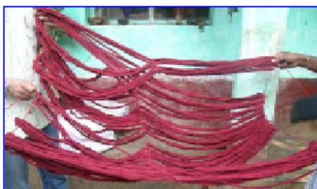
First of all two *mudas* are tied as one with rope for convenience of handling the yarn reels. The yarn from the mill is washed thoroughly in cold water.
